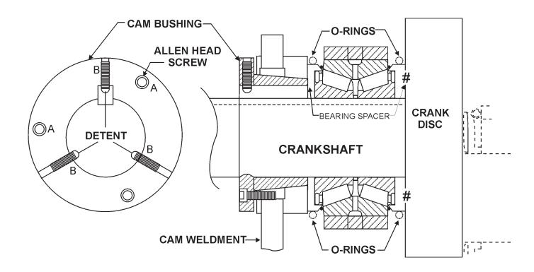
Figure 25. Bearing/Cam Bushing Installation
